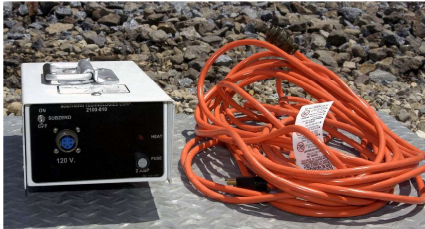
Figure 13-7 Calibrated Heat Source
